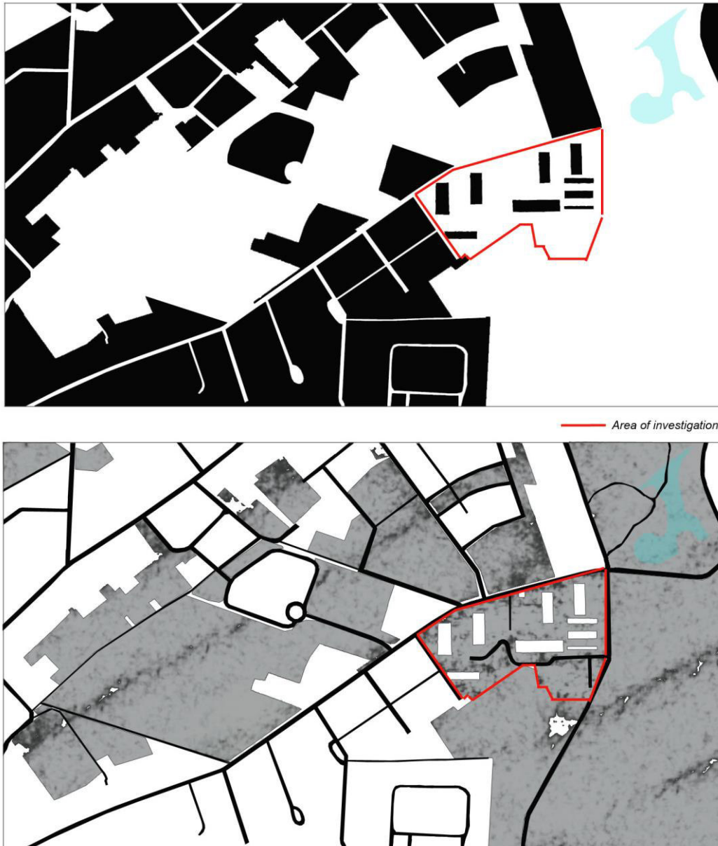
Fig. 13a and 13b: Graphic representation of solids and voids. the area that is here identified as "full" is very small compared to the "empty" but incredibly dense, as it is large buildings in line between 7 and 10 floors high.
