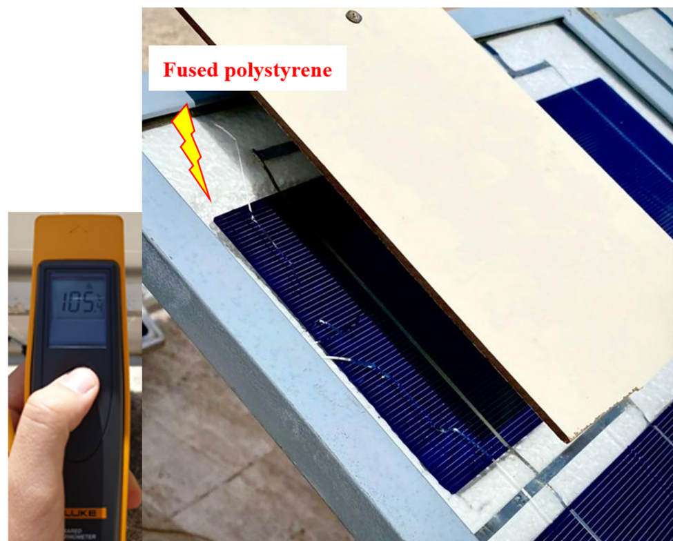
Figure 11. Some damage on the homemade submodule, when only a single PV cell has been partially shaded, and the bypass diode of the submodule intervened.
