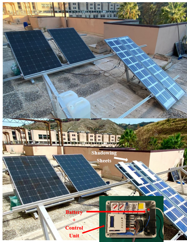
Figure 3. Some pictures describing the prototypal PV generator together with the BCU.
