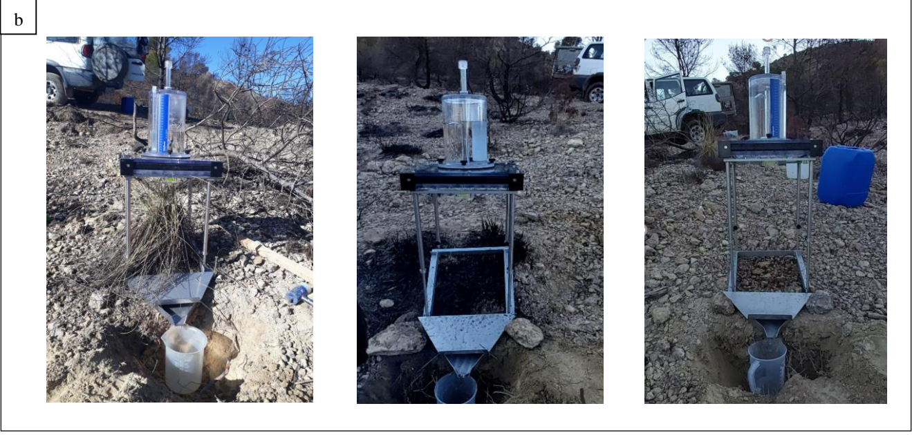
Figure 1 – Geographical location of the study area (Agramòn, Castilla La Mancha, Spain) (a), and rainfall simulations carried out under three experimental soil conditions (unburned M. tenacissima - left, burned M. tenacissima – center, and bare soil - right) (b).
