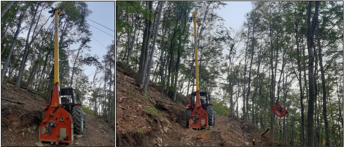
Figure 2. Valentini V 400 tractor-based tower yarder.
