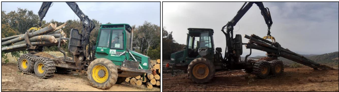
Figure 3. Timberjack 1010D clambunk skidder.
