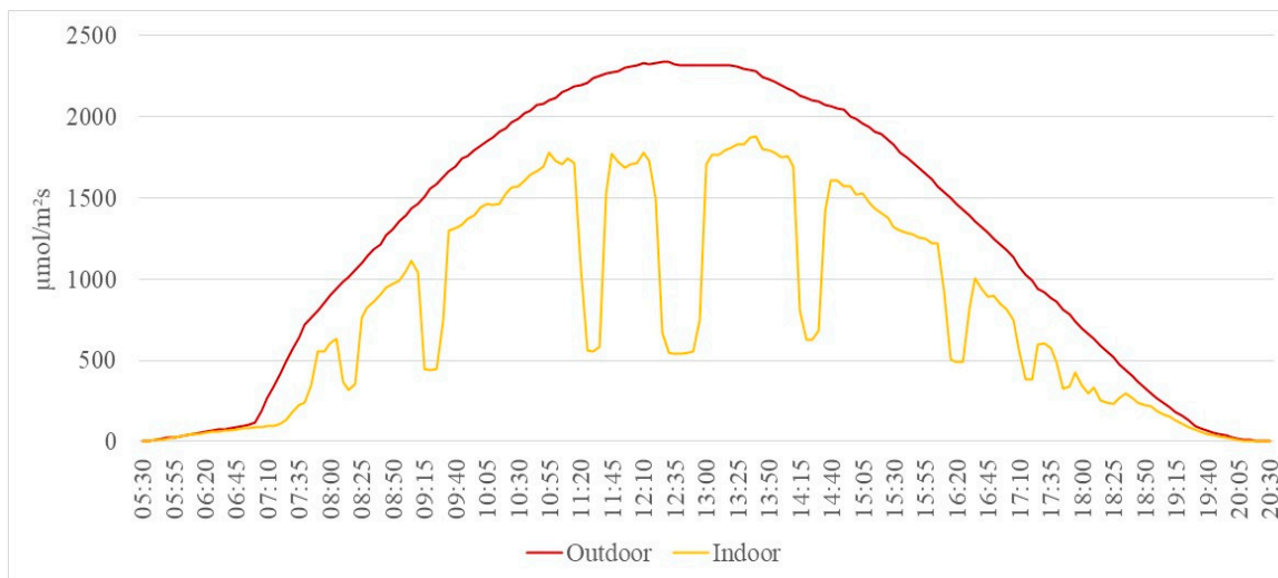
Figure 2. Hourly e-PAR values for the outdoor environment and greenhouse interior.
