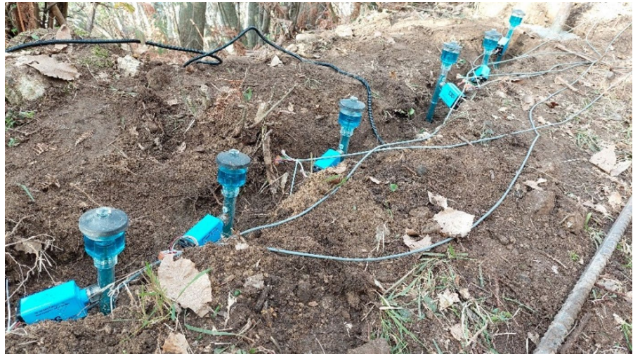
Fig. 11 Tensiometers installed in Monitoring Station N. 1
