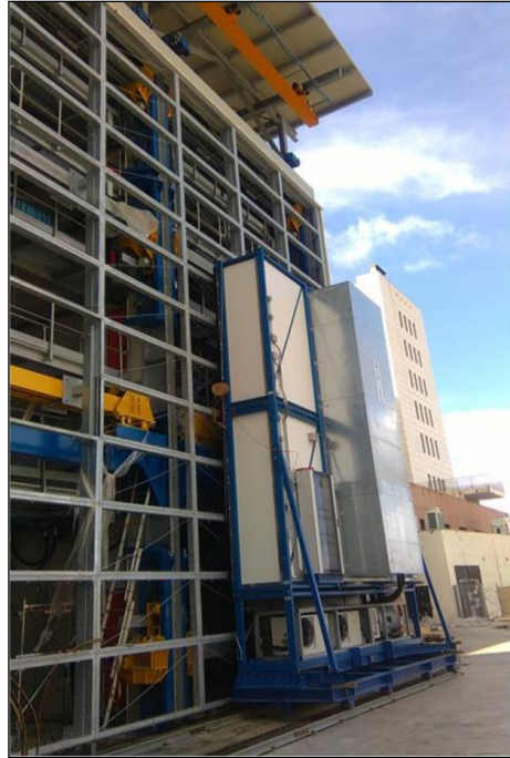
Fig. 2 - Thermal Chamber, made in accordance 15 x 12 x 4.5 m, for trying make-up with the AAMA 501.5-07 of maximum size between 170 and 200 sm "Test Method for Thermal Cycling of Exterior Walls"
