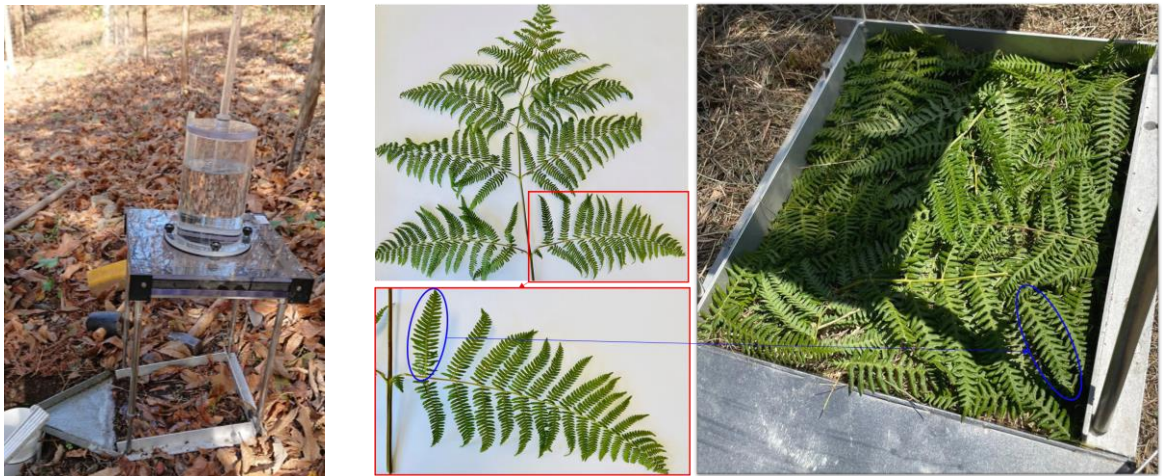
Figure A3. Measurements of soil hydraulic conductivity (using a portable rainfall simulator) and fern mulch application into the rainfall simulator at the experimental site (Samo, Calabria, Southern Italy).
