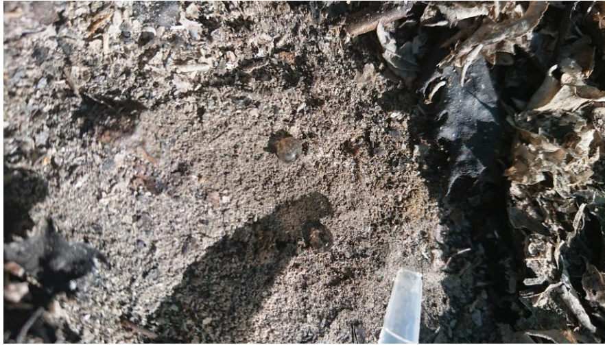
Figure A4. Measurements of soil water repellency (by the WDPT method) in the experimental site (Samo, Calabria, Southern Italy).
