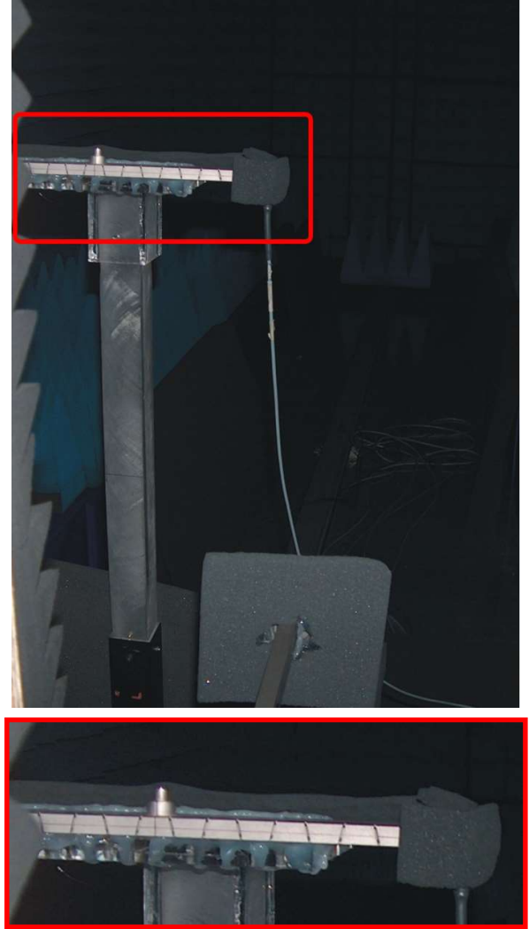
Fig. 15. Photo of the slotted-waveguide array into the anechoic chamber at University of Calabria. The rectangular waveguide used as measuring probe is also visible at the bottom.
