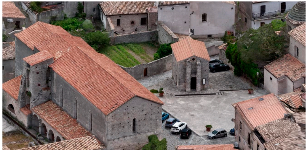
Figure 3. Textured mesh of Piazza delle Tre Chiese in Gerace (RC) obtained by integrating multiple survey techniques, including terrestrial and aerial photogrammetry and laser scanning. The church of San Giovannello is in the centre, and the convent and church of San Francesco are on the left. Image reproduced from reference [10] (CC BY 4.0).
