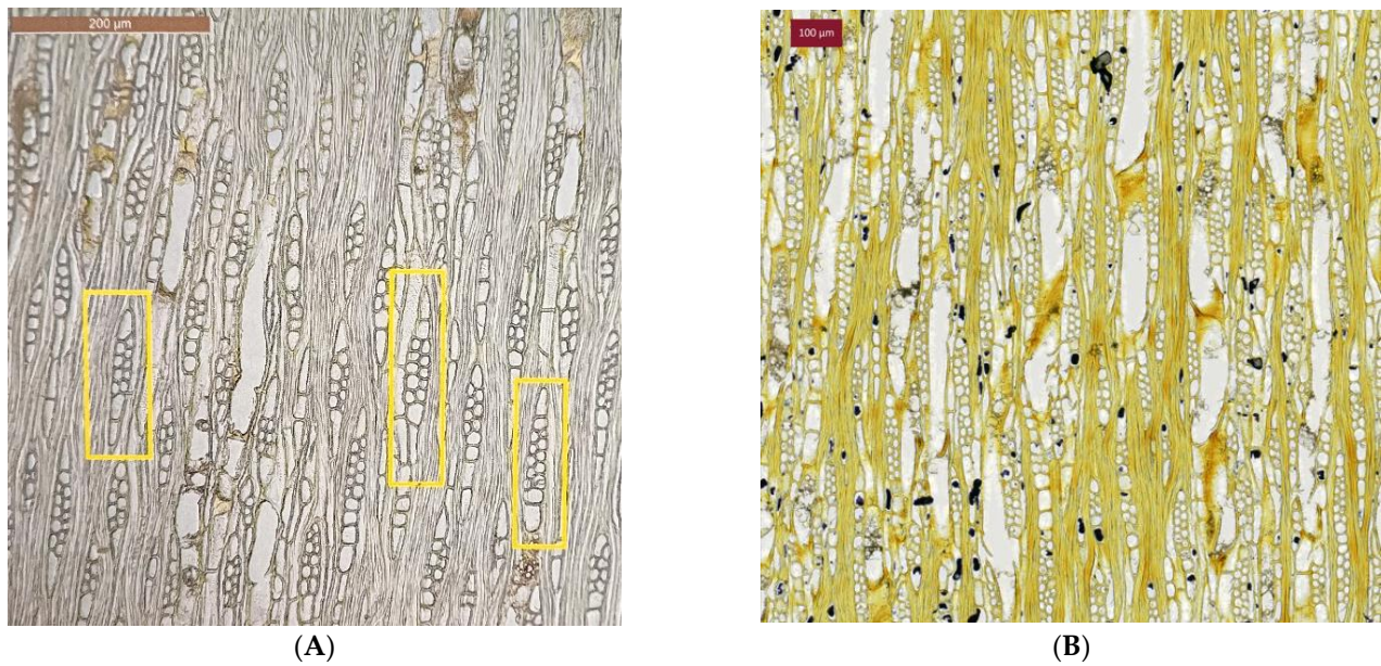
Figure 8. Sinopolese olive wood cultivar: (A) 1B sample, heartwood; (B) 15B sample, sapwood. Tangential section. Yellow boxes: ray width with one to three cells (IAWA feature 97 [26]).
