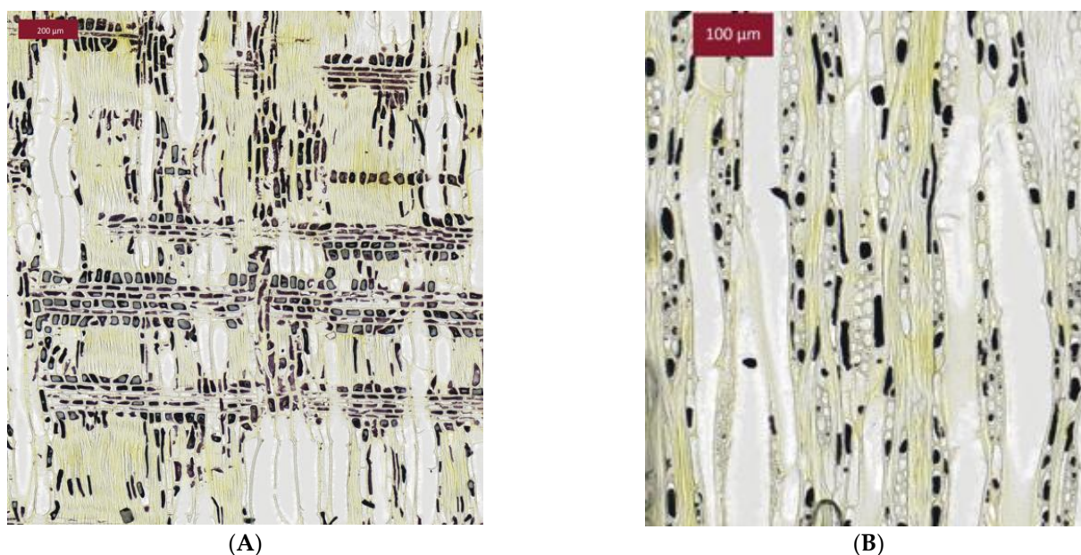
Figure 10. Starch (black spots) in Ottobratica olive wood cultivar, 5A sample, sapwood. (A) Radial section, (B) tangential section.
