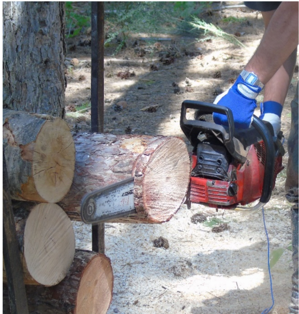
Figure 3. The noise and vibration measurements during cross-cutting operation.
