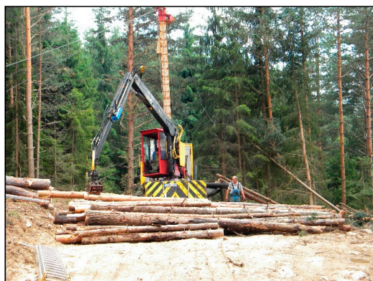
Figure 2. Koller K501 yarder during the operations: (a) view from the landing site; (b) view from the lateral yarding.
