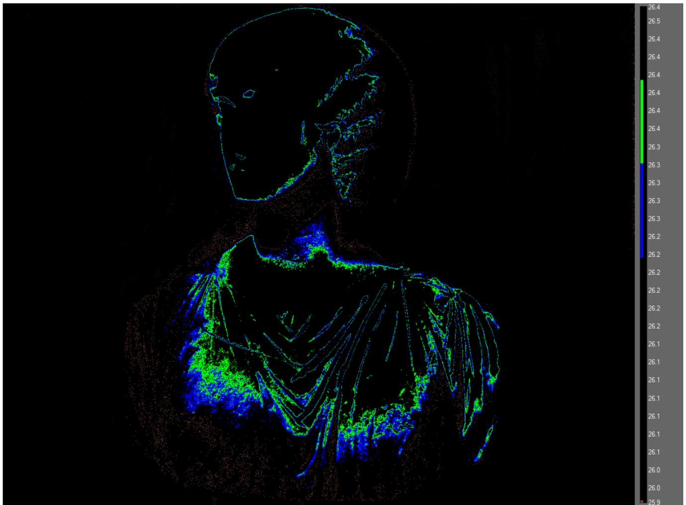
Figure 9. Classification of material alterations: pure marble (green colour); alveolised marble (blue colour); iron oxidized marble (brown colour).
