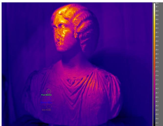
Figure 7. The chosen three circular ROIs (from bottom): Iron Oxide (in brown colour); alveolisation (in blue colour); pure marble (in green colour).
