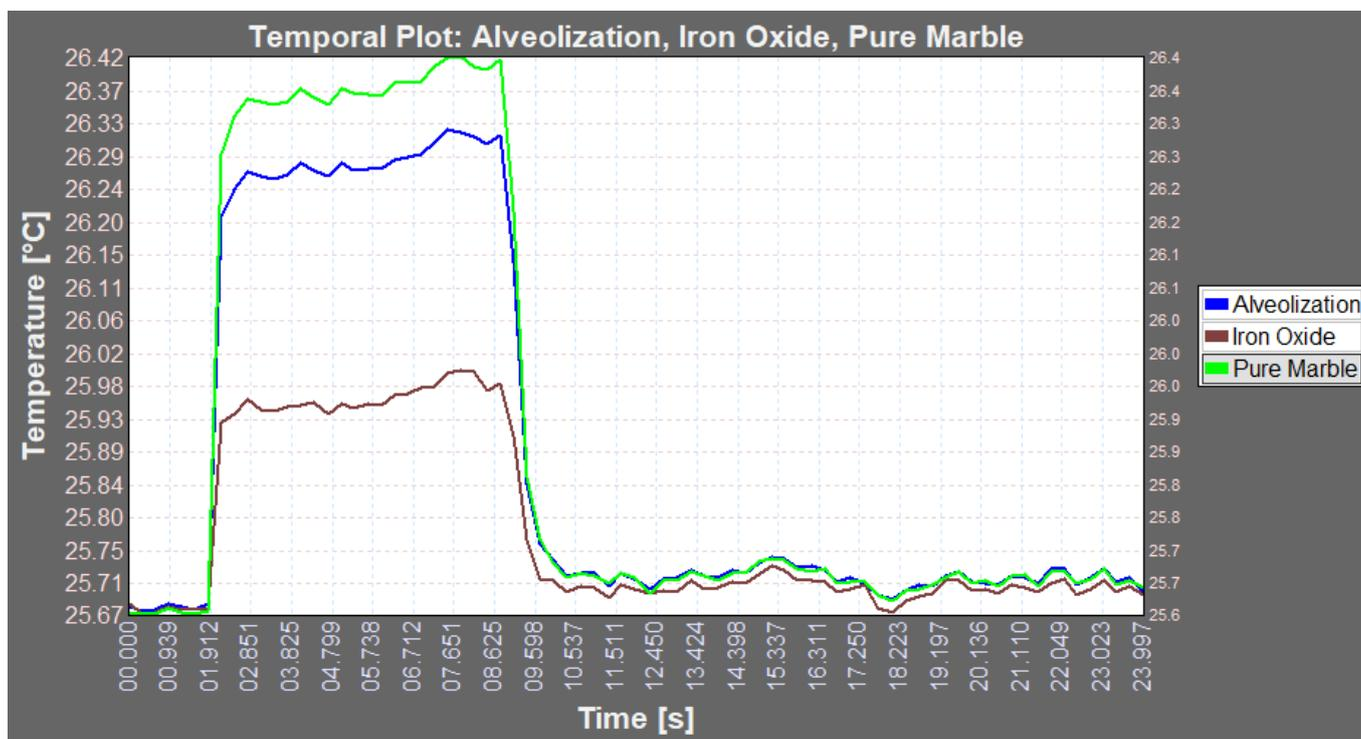
Figure 8. Plot of the thermal response of the three ROIs over time (from bottom): Iron Oxide (in brown colour); alveolisation (in blue colour); pure marble (in green colour).
