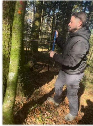
Figure 11: Coring of trees through the use of the Pressler's increment borer.
