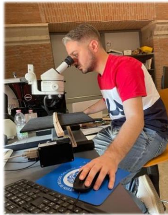
Figure 12: Tree rings analyses using the LINTAB-measurement equipment.
