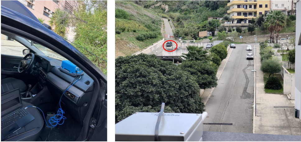
Fig. 3.8: Testbed in the campus premises: OBU mounted on board (left) and RSU covering the area where the equipped vehicle (the one within the red circle) moves (right).
