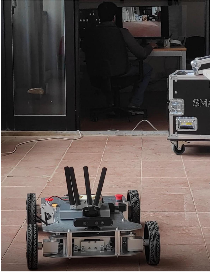
Fig. 4.7: PoC teleoperation setup: robot and driving station used over the 5G-SA testbed.
