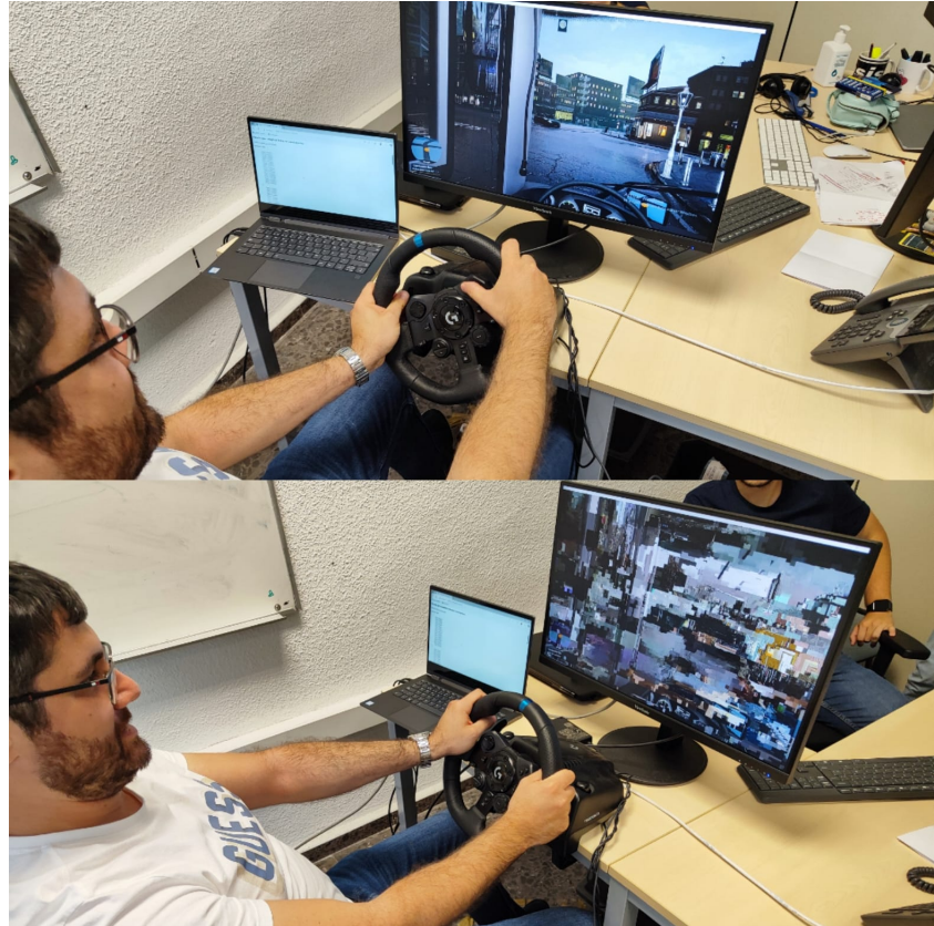
Fig. 4.2: ToD operator workstation used during the research stay at UPM, including the driving interface and the visual feedback supporting remote vehicle control.
