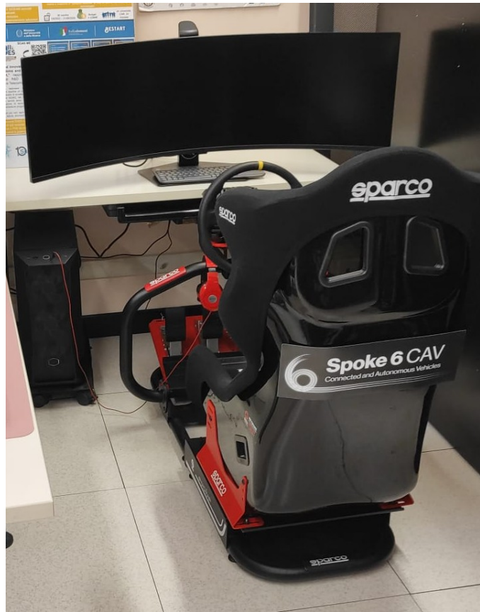
Fig. 4.8: Remote driving station used over the 5G-SA testbed.
