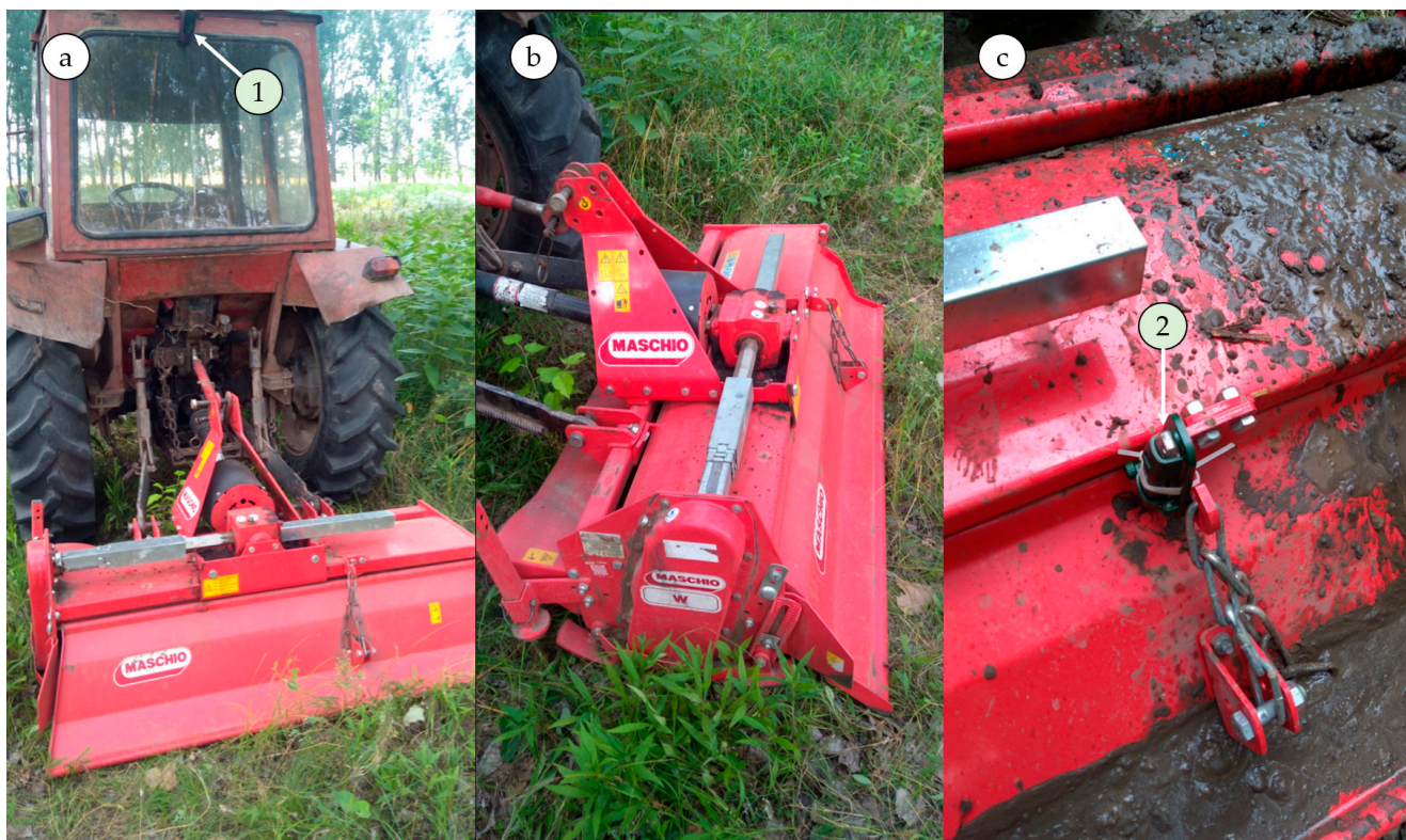
Figure 2. Configuration of the equipment taken into study: (a) the farm tractor equipped with the rotary tiller showing the location of the handheld GNSS receiver (1); (b) the rotary tiller observed in the study, (c) placement of the triaxial accelerometer (2) on the rotary tiller.
