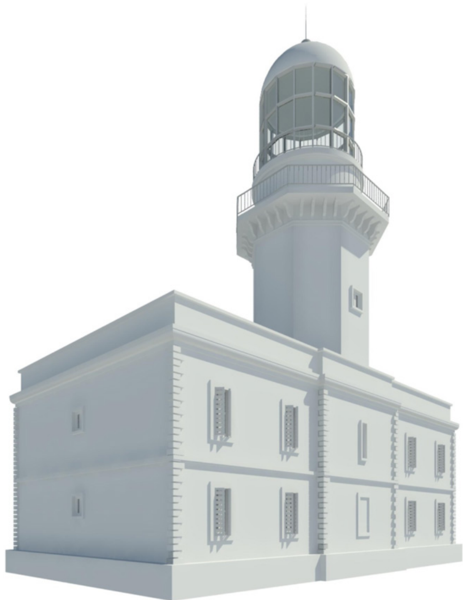
Fig. 40. Parametric model of the Capo Colonna lighthouse created using the design model of the Italian lighthouses.
