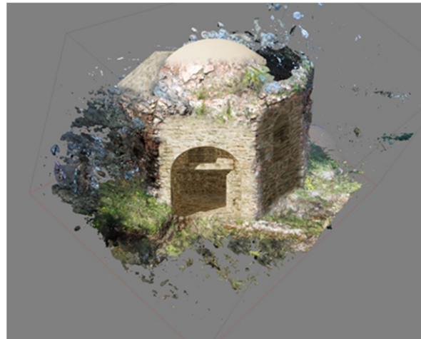
Figure 11. Overlap between BIM and dense cloud.
