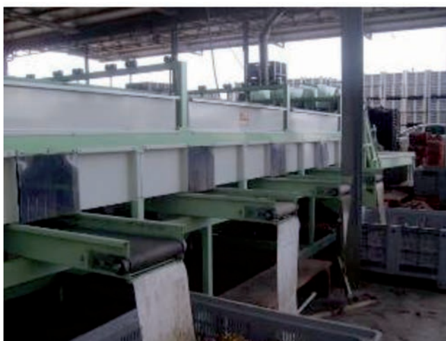
Figure 1. Onion grader with inclined belts.
