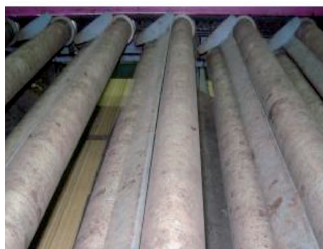
Figure 2. Onion grader with rollers.
