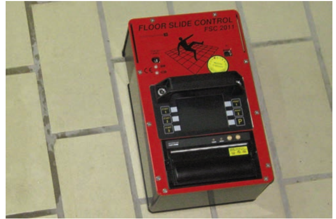
Figure 2. Survey of coefficient of friction on the floor by the Tortus digital tribometer FSC 2011.
