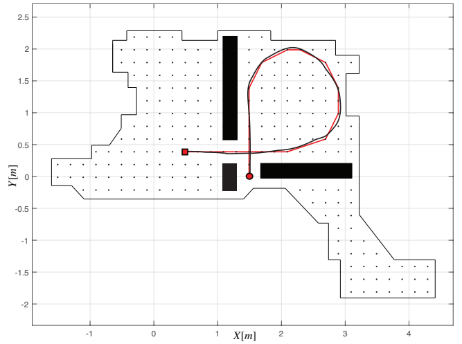
Fig. 6. 2D operating environment with obstacles (black boxes). Red line denotes the optimal feasible trajectory connecting starting (square) and ending (circle) points. Black solid line represents tracked mobile robot trajectory.
