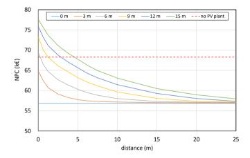
Figure 17. NPC vs building distance, for different heights
