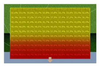
**Figure 12**. Shadow distribution and irradiation percentage on panels
