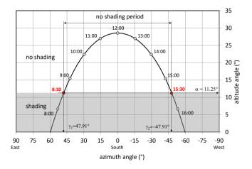
**Figure 2**. Sun path referring to 21st December, with panel shading hours indication
