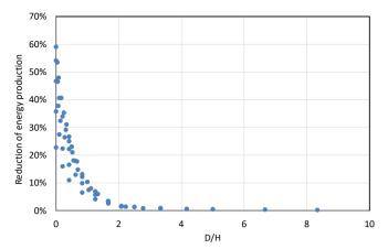
**Figure 16**. Reduction of yearly energy production vs. distance/height
