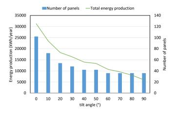
**Figure 6**. Produced energy and number of panels vs. tilt angle
