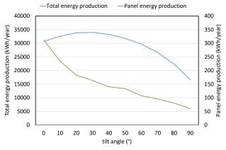
Figure 7. Energy production vs. tilt angle
