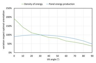
**Figure 8**. Energy production, total and referred to unitary occupied surface, vs tilt angle
