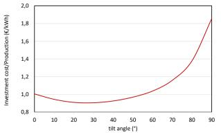
Figure 10. Investment cost/production vs. tilt angle
