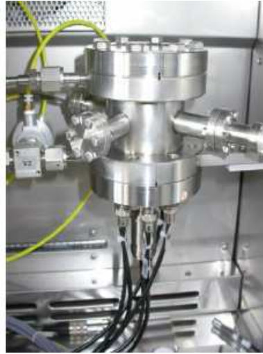
Fig. 3. 11 Stainless steel chamber used for gas sensing test (Enea Portici Research Center).
