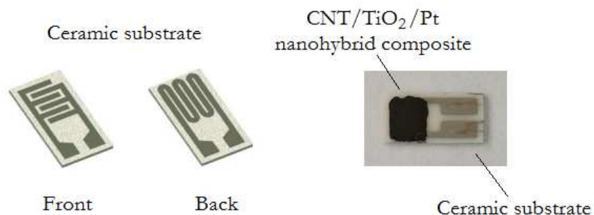
Fig. 3. 19 (a) Ceramic substrate provided with comb-like Pt-electrodes in front and a Pt-heater on the back; (b) CNT/TiO 2 /Pt sample deposited on the ceramic substrate.
