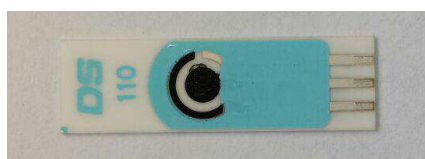
Fig. 3. 24 CNT/TiO 2 /Pt hybrid deposited on a commercial electrode.
