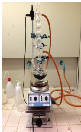
Fig. 2. 45 Carbon nanotubes functionalization system.
