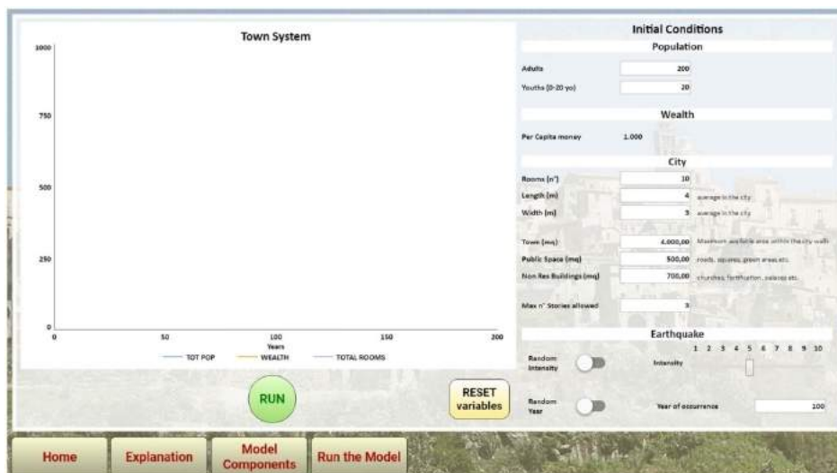
Fig. A5.1 – On the right an interface allows to setup the initial conditions of the model. Variables can be customised at level of town. The occurrence and intensity of the earthquake can be established or left random. Drawing by Guglielmo Minervino
