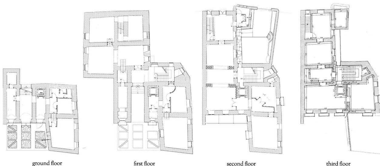
Fig. A1.26 –Plans of a case palizziata in Paola. It is evident the difference in floors perimeter as result of the merging of multiple properties and expantions. Drawing elaboration by Guglielmo Minervino
