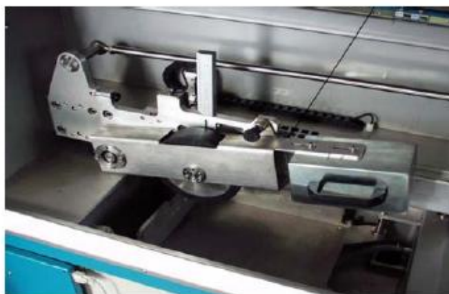
Figure 2.30 Hamburg wheel tracking tester Laboratory tests
