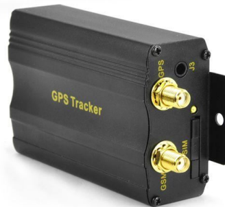
Figure 10.6: Example of TK103 GSM/GPRS/GPS Tracker device for vehicles.
