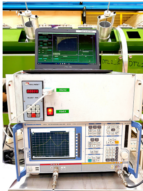
Fig. 3.7: Setup used for bead pull measurements. VNA and motor are controlled through a LabView script that acquires and saves the measures.
