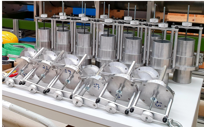
Fig. 3.11: Post-couplers (lower photo side) and tuners (upper photo side) used for the RF tuning of the ESS DTL tank 2 cold model.
