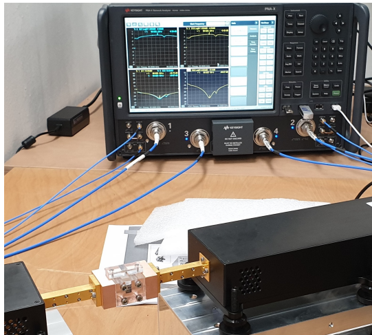
Fig. 10.5: Photo of the experimental setup used to measure S-parameters of the structure: the manufactured woodpile waveguide and rectangular waveguide to EBG waveguide transition have been connected to the mm-wave extension heads of the Agilent PNA-X Vector Network Analyzer.
