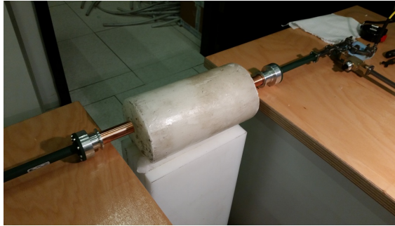
Fig. 5.45. Setup with paraffin wax cylinder between horns
