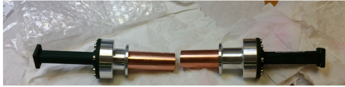
Fig. 5.24. The final assembly of the horn antennas
