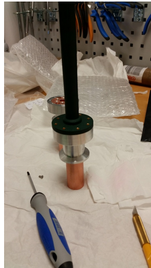
Fig. 5.23. Antennas connection to the transition "in waveguide"
