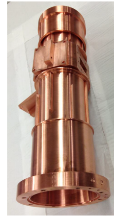
(b) Oxygen free high conductivity copper FPT plasma chamber
