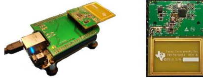
Fig. 10.1: The BeagleBone with the RFID Adaptor Board and the Texas Instrument's TRF7970ATB RFID module
