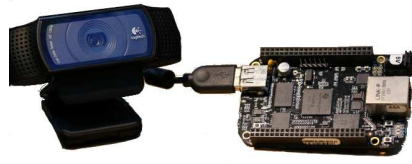
Fig. 10.2: The BeagleBone and the Logitech C920 webcam
