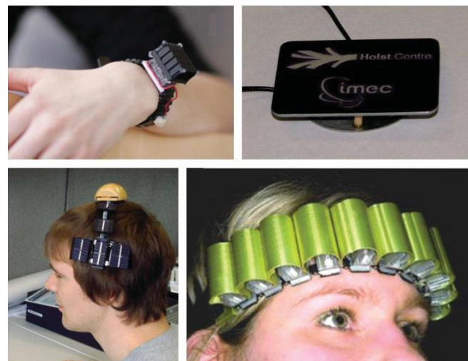
Fig. 1.5 Wearable Thermoelectric Energy Harvesting used for measurements of thermal properties of humans and power generation on people at different ambient conditions[15]
