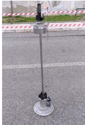
Fig. 5.1 Light Weight Deflectometer (LWD) used in the on-site experiments.
