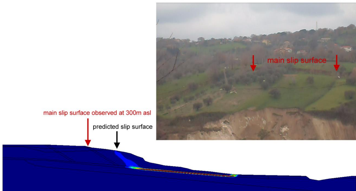
Fig.4.51- A different slip surface than that observed one (indicated by red arrows) is found in the second analysis
