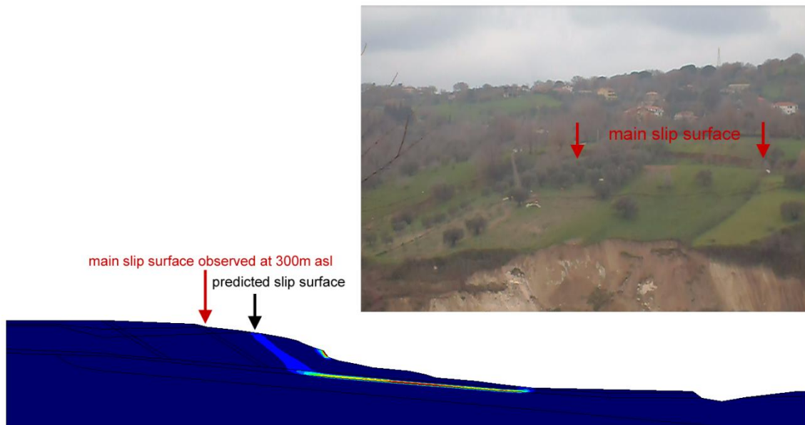
Fig.4.52 - A different slip surface than the observed one (indicated by red arrows) is found in the third analysis
