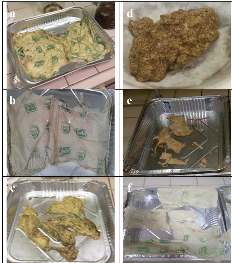
285 Figure 2. Digested compostable bags visual inspection; a) raw - mesophilic conditions – 15 days, b) 286 raw - mesophilic conditions – 30 days, c) raw - thermophilic conditions – 15 days, d) raw - 287 thermophilic conditions – 30 days; e) NaOH pre-treated - mesophilic conditions – 15 days, f) pre- 288 digested - mesophilic conditions – 15 days.
