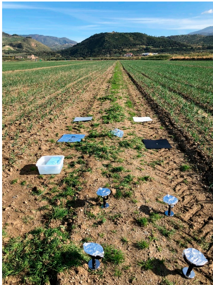
Figure 4. The temperature reference targets used during thermal unmanned aerial vehicle (UAV) surveys in an onion crop field in Calabria (Italy) (photo taken by the authors).
