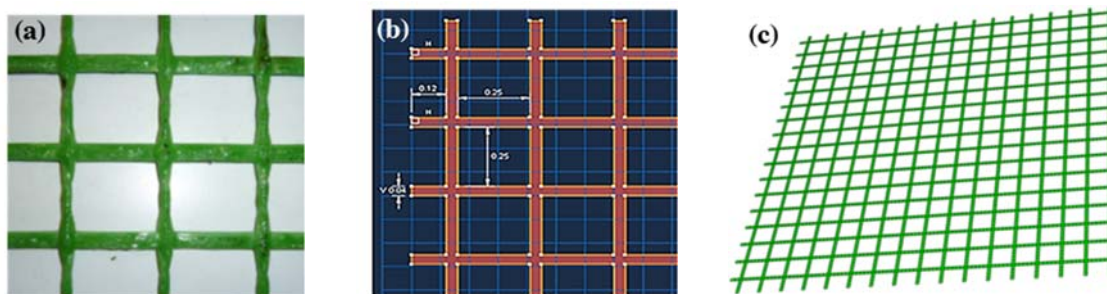
Figure 3. Glass fibre grid layer: a) plane view; b) open meshes dimension; c) mesh model
