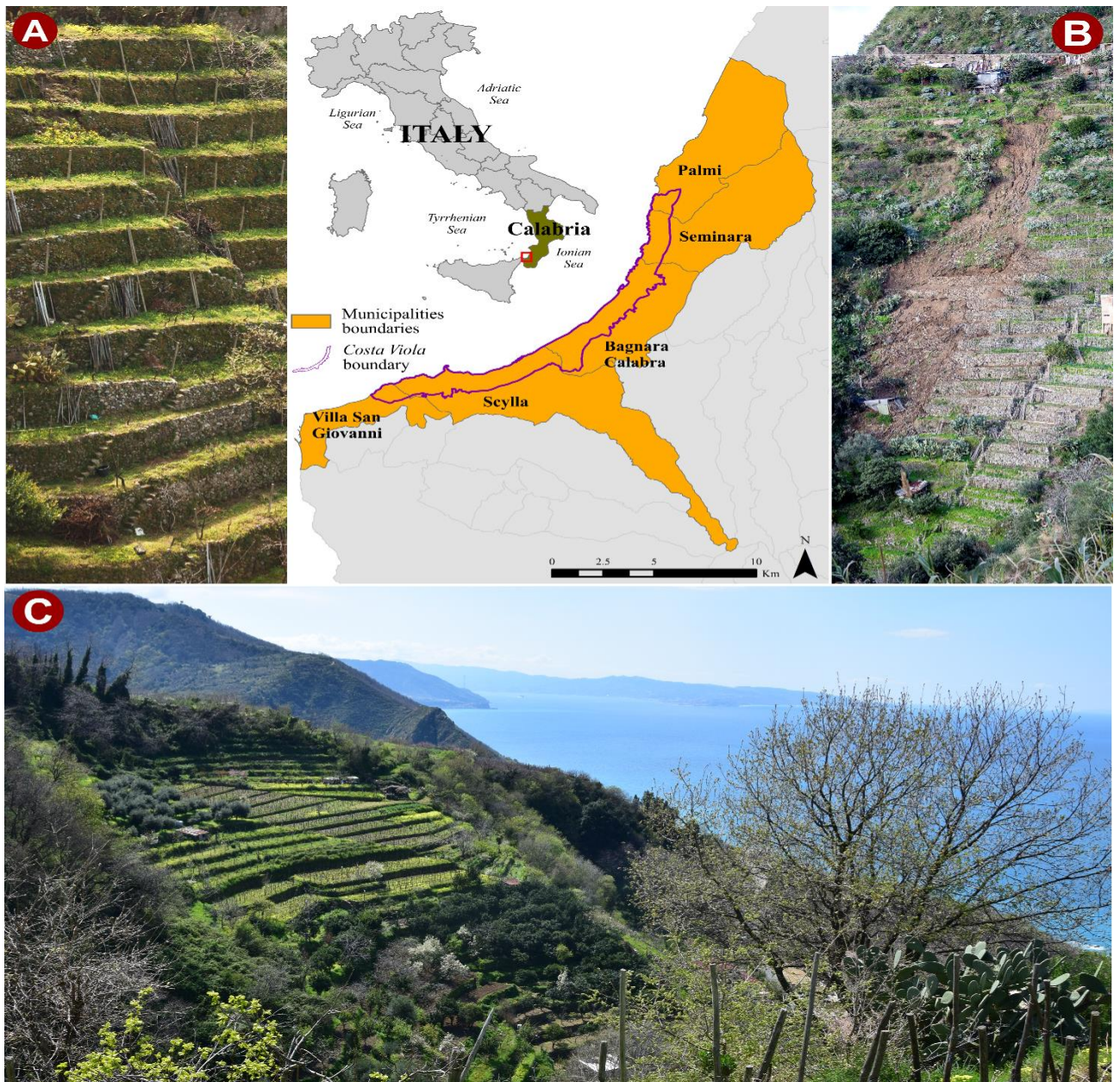
Fig. 1 – Geographical localisation of the study-area, Costa Viola . Example of the traditional cultivated agricultural terraced landscape of Costa Viola characterised by dry-stone retaining walls (A); a recent shallow landslide (December 2015) with the initiation point located in an abandoned terrace and interesting a cultivated one (B); panoramic view of a typical terraced area (C).
