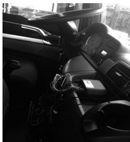
Figure 1. Installing the GPS/GSM black-box unit.
