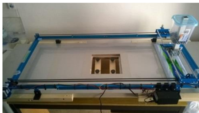
Figure 1 - Automated mechanical system for the simulation of the tile cleaning
