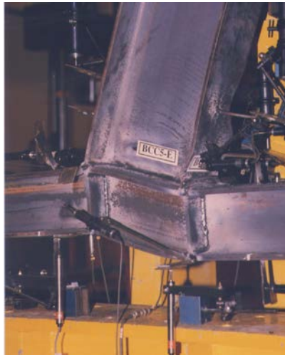
Fig. 6. Specimen BCC5-E at collapse.
