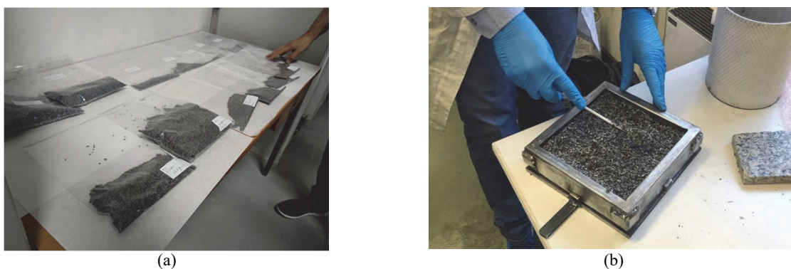
Fig. 4. Testing in ENEA and UNICAL Diatic Laboratory (Lucanto and Procopio, 2019) (a) represent the samples of the virgin separated from the metallic matrices (b) represent the first test of forming the in the mold for the press and the realization of the thickness block for the green parking
