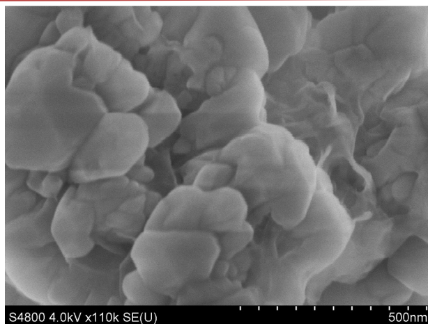
Fig. 3. SEM graph of sample heat treated at 1550 °C in N 2 -atmosphere.
