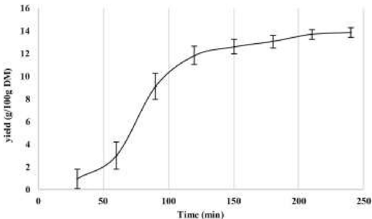
Fig. 2. Extraction yield vs extraction time at the central point of the response surface design experimental condition pressure 200 bar temperature  $55 \text{ }^{\circ}\text{C}$  and co-solvent EtOH 90%.
