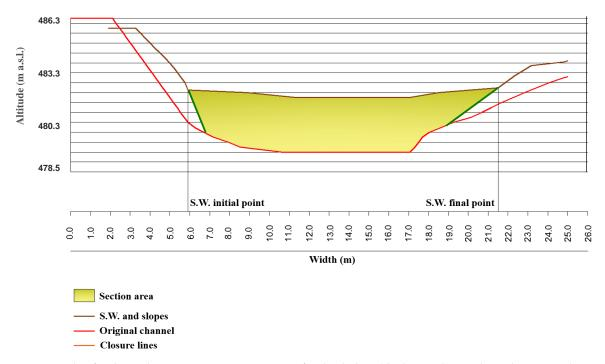
**Figure 3.** Example of a channel cross section in proximity of a check dam (the brown line is the sediment wedge profile, the red line the channel profile, and the green line is the hypothesized bank profile close to the sediment wedge; the yellow-shadowed line is the area of the channel cross section).
