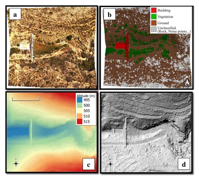
**Figure 4.** Cartographic products obtained in the aerophotogrammetric survey for Conejo (number 1) check dam (Sierra de Los Donceles forest, Castilla La Mancha, Spain): (**a**) 3D point cloud; (**b**) Classified point cloud; (**c**) Digital Terrain Model (DTM); (**d**) Shaded DTM.
