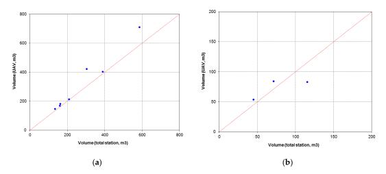
**Figure 6.** Scatter plots of sediment wedge volumes measured by the aerophotogrammetric and topographic methods for ten check dams (Sierra de Los Donceles forest, Castilla La Mancha, Spain) (**a**), larger check dams,  $V > 100 \text{ m}^3$ , (**b**), smaller check dams,  $V < 100 \text{ m}^3$ .
