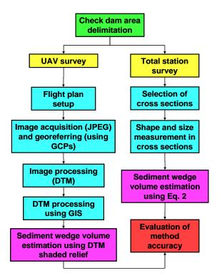
**Figure 2.** Workflow of the process for calculating sediment wedge behind check dams using aerophogrammetric (by UAV) and topographic (by total station) methods.
