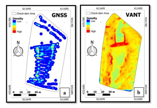
**Figure 7.** Point clouds obtained by the topographic (**a**) and aerophotogrammetric (**b**) methods for the Palomar check dam (Sierra de Los Donceles forest, Castilla La Mancha, Spain).
