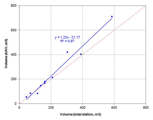
**Figure 9.** Regression of sediment wedge volumes estimated by the aerophotogrammetric and topographic methods for ten check dams (Sierra de Los Donceles forest, Castilla La Mancha, Spain).
