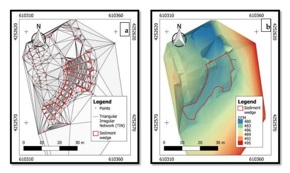
**Figure 5.** Points and related Triangular Irregular Network (TIN, (**a**) as well as Digital Terrain Model (DTM, (**b**) obtained in the topographic survey for Grillo (number 3) check dam (Sierra de Los Donceles forest, Castilla La Mancha, Spain).
