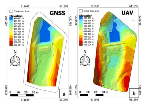
**Figure 8.** Digital Terrain Models (DTMs) obtained by the topographic (**a**) and aerophotogrammetric (**b**) methods for the Palomar check dam (Sierra de Los Donceles forest, Castilla La Mancha, Spain).
