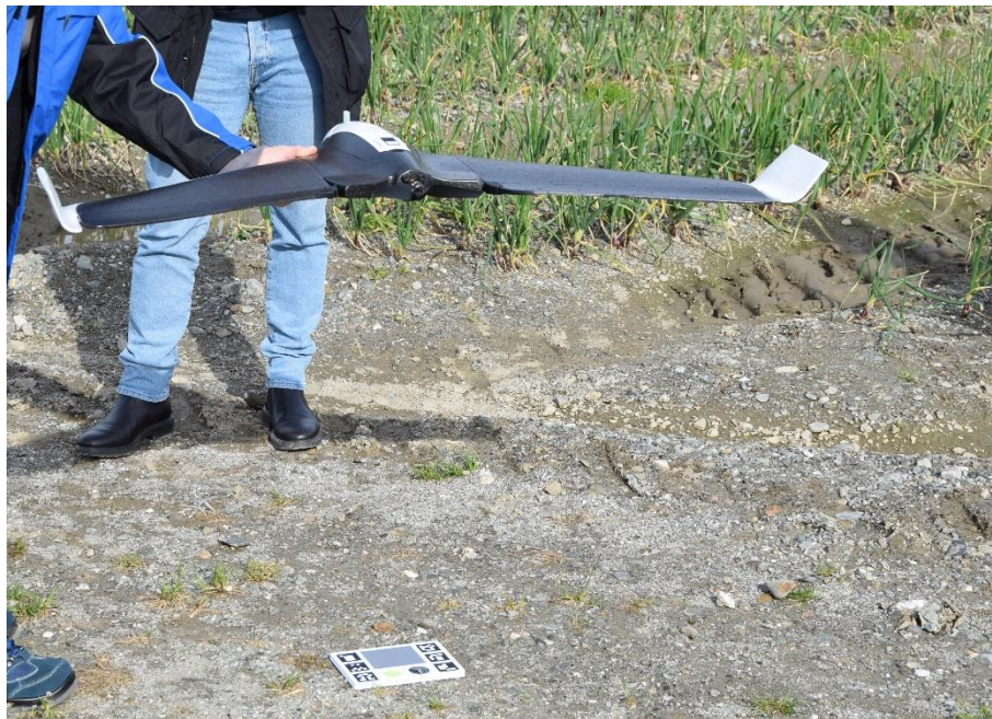
Figure 6.3 The Parrot Disco-Pro AG fixed-wing unmanned aerial vehicle (UAV) during the pre-flight calibration using the Parrot Sequoia calibration target ( source , Messina et al., 2020c).
