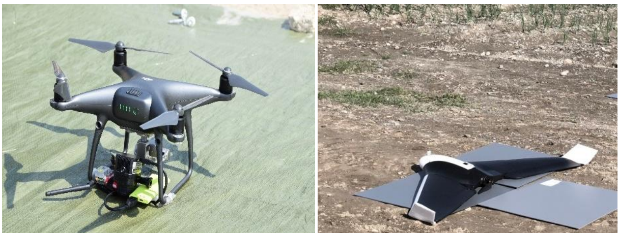
Figure 5.6 The quadcopter DJI Phantom 4 equipped with the thermal camera FLIR Vue Pro R 640 (on the left) and the fixed-wing Parrot Disco-Pro AG equipped with the multispectral camera Parrot Sequoia (on the right) ( source , Messina et al., 2019).
