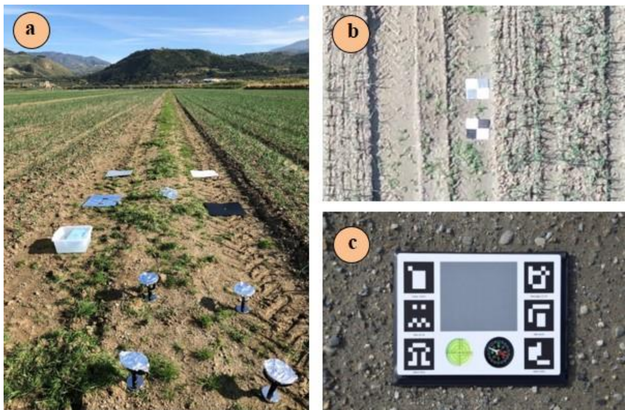
Figure 5.9 (a) Temperature reference targets used during thermal surveys. (b) Thermal (above) and multispectral (below) targets are used as ground control points (GCPs) in the onion field. c The Parrot Sequoia calibration target ( source , Messina et al., 2019).
