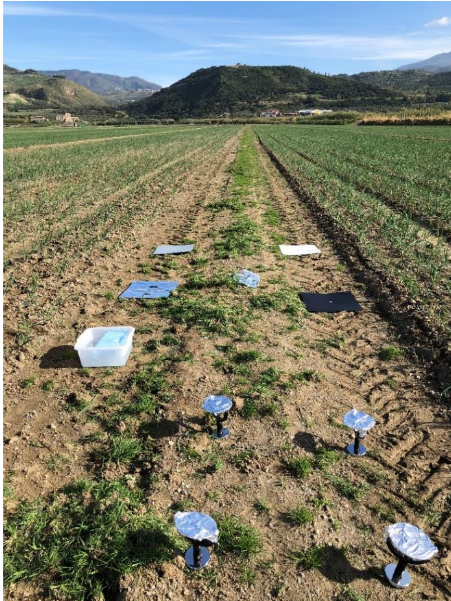
Figure 5.2 The temperature reference targets used during thermal unmanned aerial vehicle (UAV) surveys carried out in an onion crop field in Calabria (Italy) ( source , Messina and Modica, 2020b).
