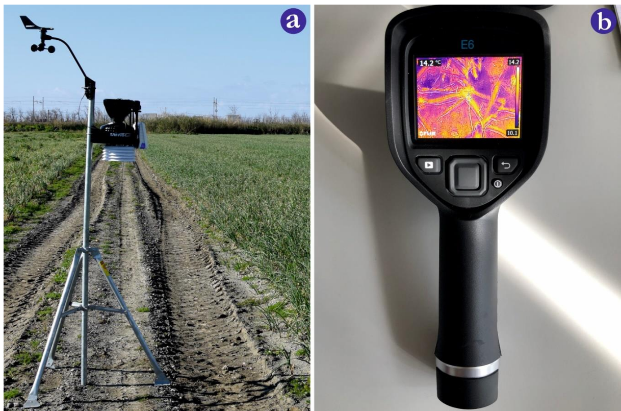
Figure 5.4 (a) The weather station used during the thermal surveys carried on an onion field and (b) the handheld infrared thermometer (model FLIR E6) used to measure the temperature of reference surfaces ( source , Messina and Modica, 2020b).
