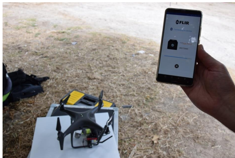
Figure 5.8 FLIR Vue Pro APP used to set the thermal camera FLIR Vue Pro.
