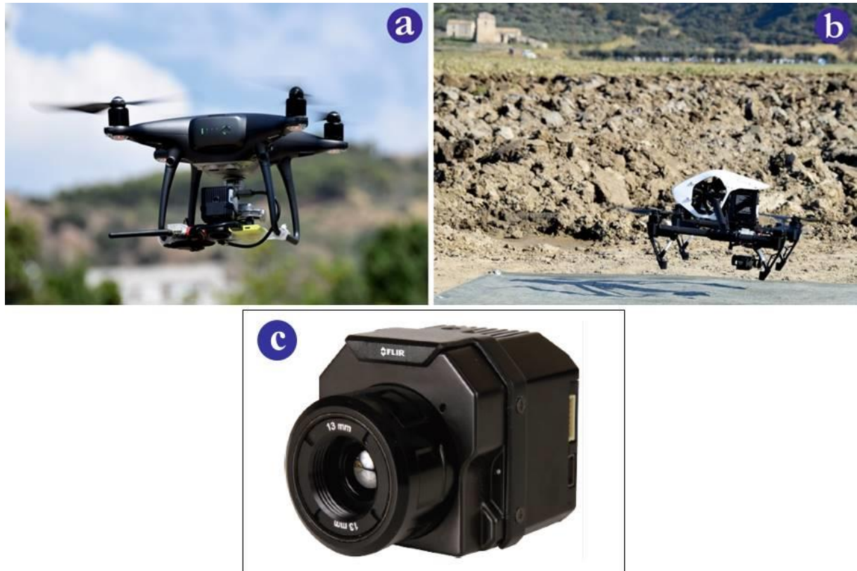
Figure 5.1 DJI Phantom 4 Pro (a), (b) DJI Inspire 1, both equipped with a FLIR Vue Pro R 640 uncooled thermal camera (c) ( sources (Messina and Modica, 2020b) and flir.it).
