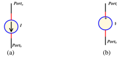
Fig. 12. Equivalent outputs of current (a) and voltage (b) signals when applied to a circuit.
