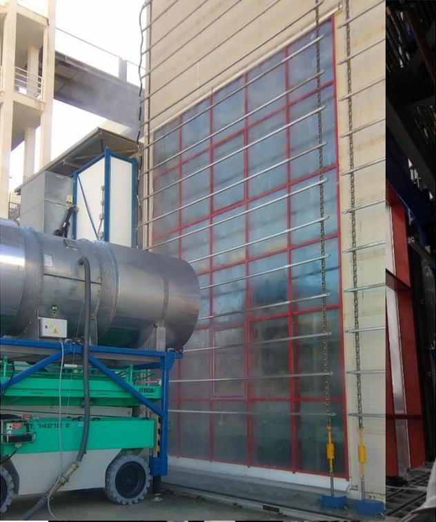
Fig 1. Mock-up of transparent façade tested
