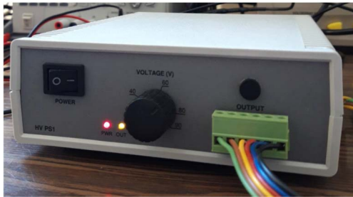
Fig. 11. Front panel of a constructed and assembled power supply for the impulse generator board.
