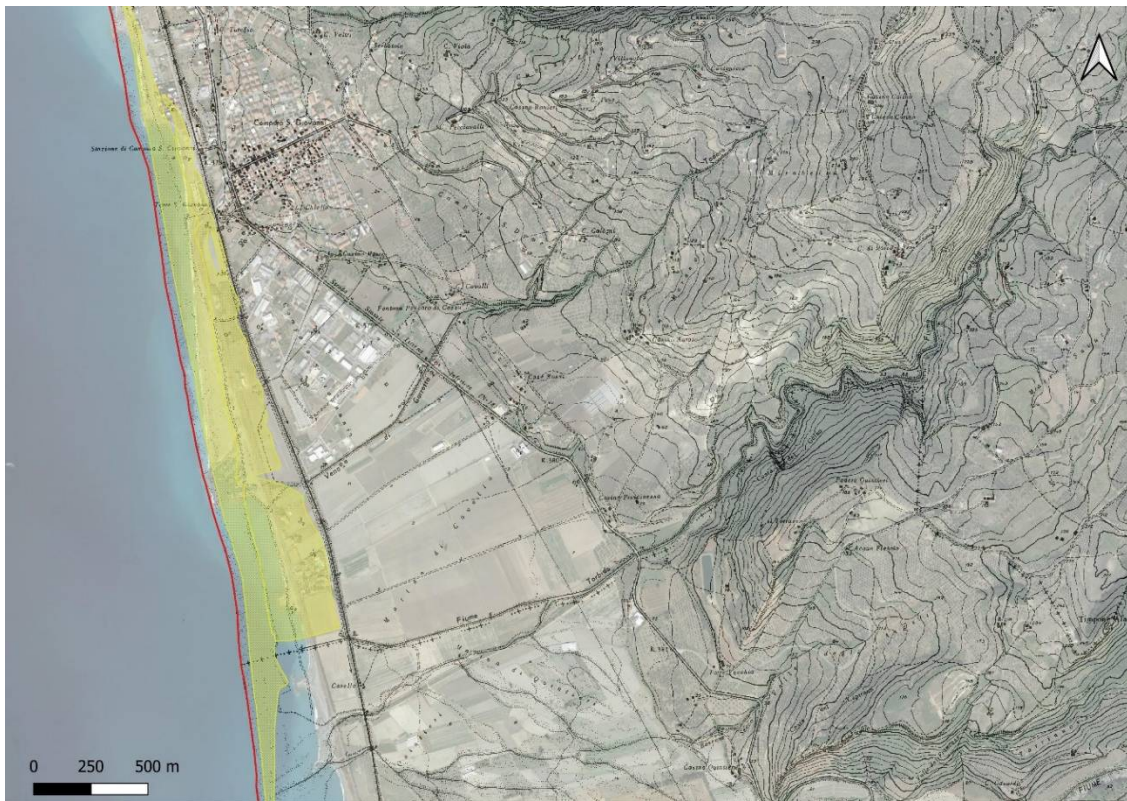
Figure 4. Amantea: overlap between CASMEZ cartography and most recent Google satellite image. Legend: red line = shoreline of 1954; yellow dotted area = dune systems of 1950s.
