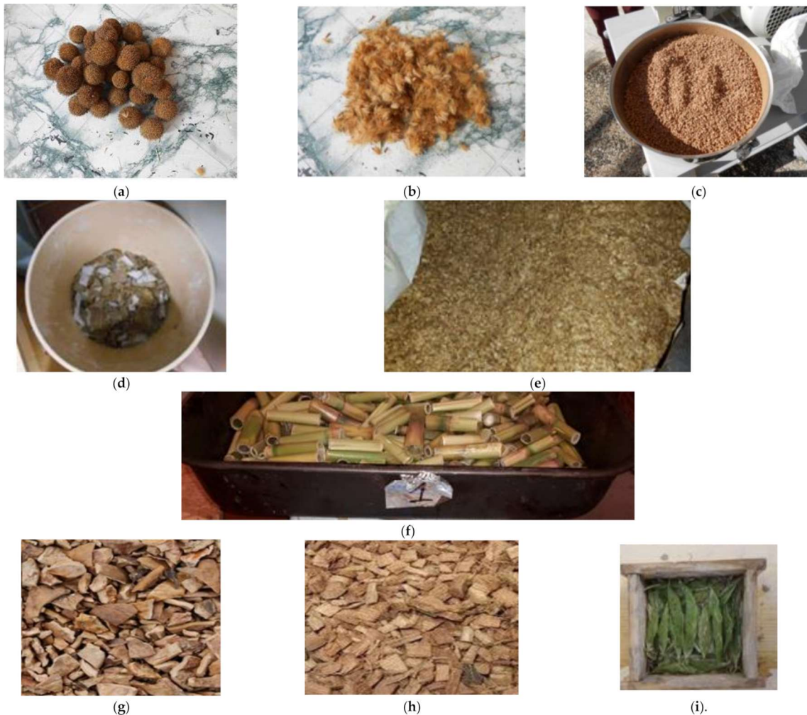
Figure 2. Natural/waste materials: (a) Desiccated platanus acerifolia fruits; (b) Smashed desiccated platanus acerifolia fruits; (c) Triturated cork plugs; (d) Water-soaked cardboard; (e) Coffee parchment skin; (f) Chopped cane stalks (g) Almond and nut shells; (h) Coconut shells; (i) Bean and pea pods.
