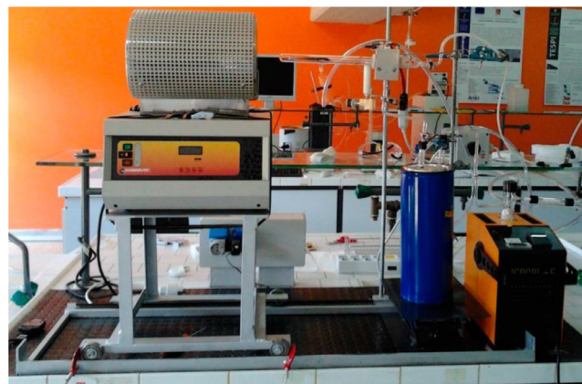
Fig. 1. The examined pyrolysis reactor.
